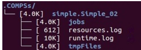
Figure 8: Structure of the logs folder for the Simple java application in info mode
