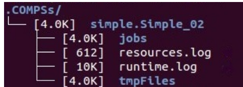
Figure 5: Structure of the logs folder for the Simple java application in info mode
